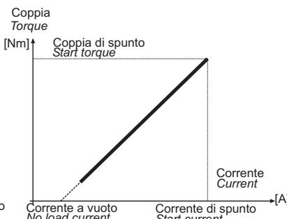
With a D.C. motor, the rotational speed is a linear function of the torque. In the same way, the absorbed current is also a linear function of the torque
