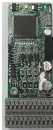
Multi-function incremental PG card EC-PG505-12
